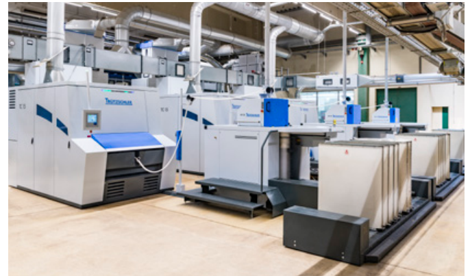
The ideal solution for rotor spinning: IDF 2 with rectangular can changer
