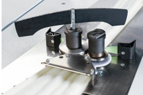
The optimised DISC LEVELLER with new quick release fastener and drive technology SERVO DRAFT are the heart of the autoleveller draw frame.
