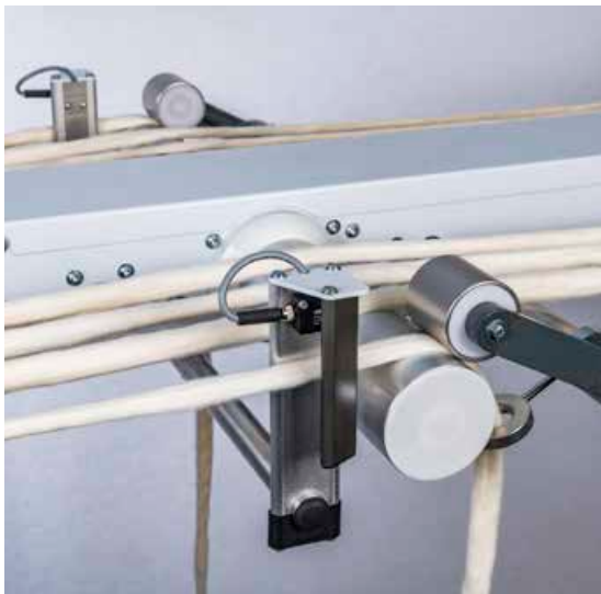
The Truetzschler breaker draw frames are also equipped with SMART sensors for individual sliver monitoring.
