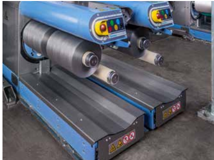
4 yarn ends with FW51 2-end winders for perfect bobbins
