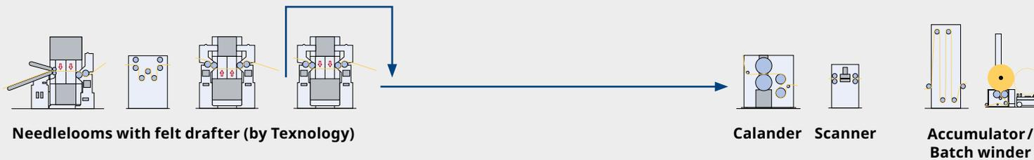
Needle-punching / finishing / winding
