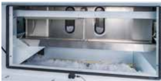
The new pan weigher with 50% increased weigh pan volume
