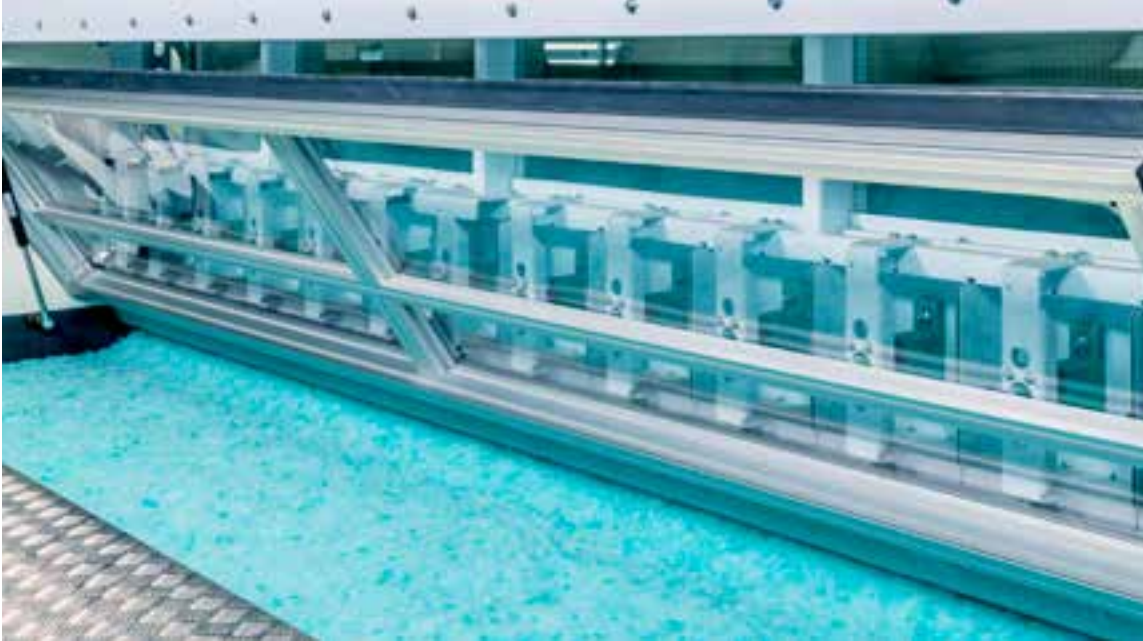
Homogeneous fiber web via TWF-TF.
