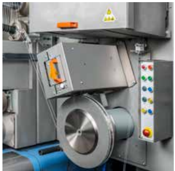
The core of BCF spinning: HPc texturing nozzle and cooling drum
