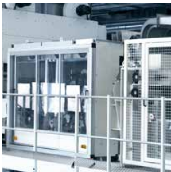
Airlay card: especially for increased weights of hygiene products
