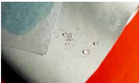
Nonwoven with hydrophilic (left) or hydrophobic finishing (right)
