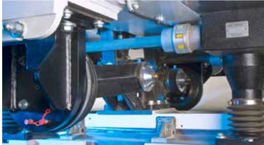
Patented, wear-free swivel bearings reduce maintenance and thus operating costs.
