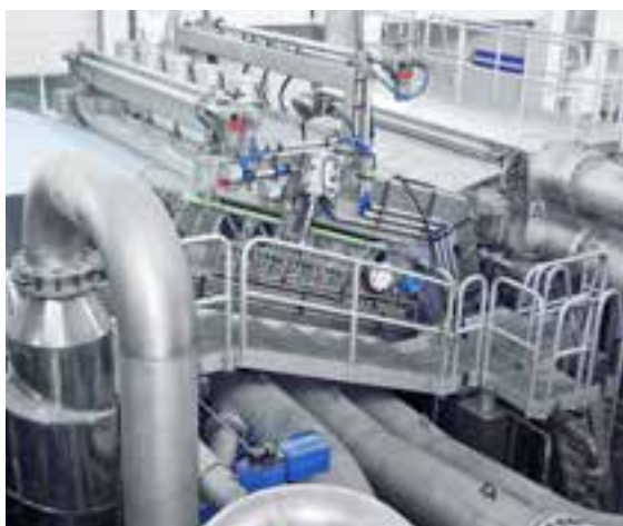
Headbox of HydroFormer
