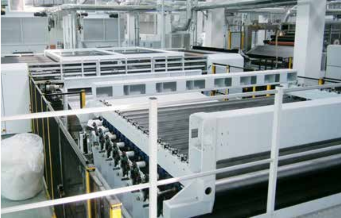
High-performance crosslapper with web drafter
