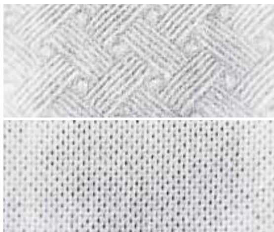
Structured (top) and perforated nonwoven (bottom)
