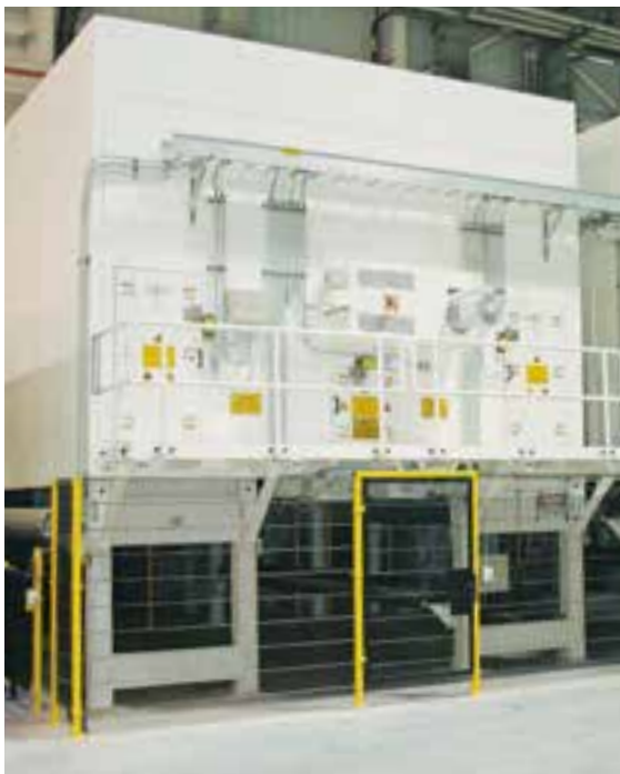
\Omega -dryer in a spunbond line
