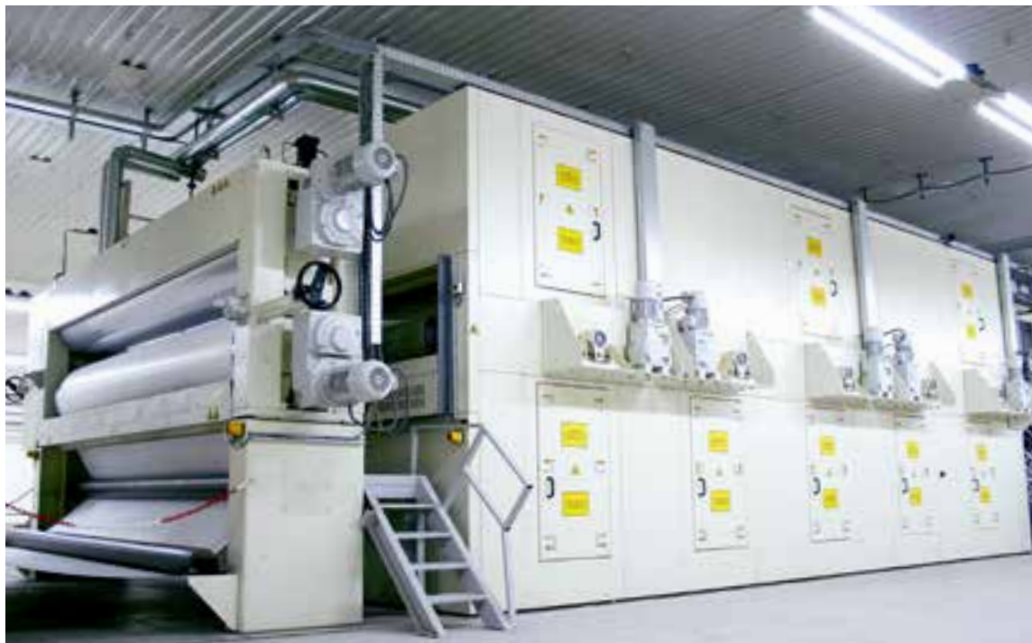
Calender and multi-drum dryer for roofing membranes
