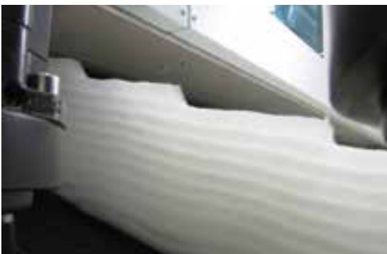
Web layer edges positioned precisely on top of each other result in reduced edge trims and thus optimal material utilisation.
