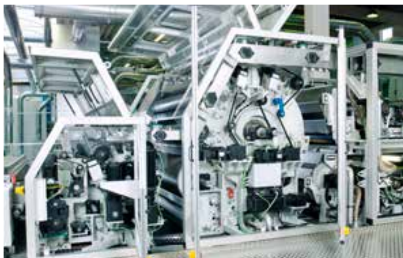
Clean card concept: Within shortest time, all maintenance points of the roller card are perfectly accessible.
