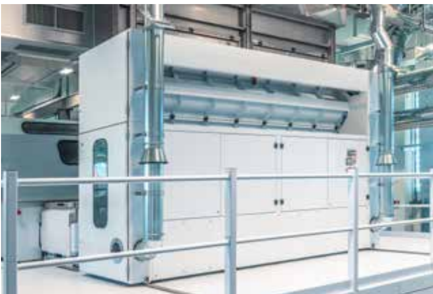
Tuft feeder TWF-TF with belt weigher and roller card
