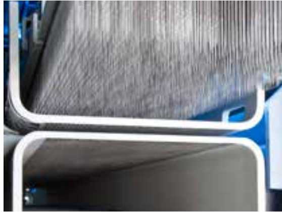
Quick replacement of needle boards
