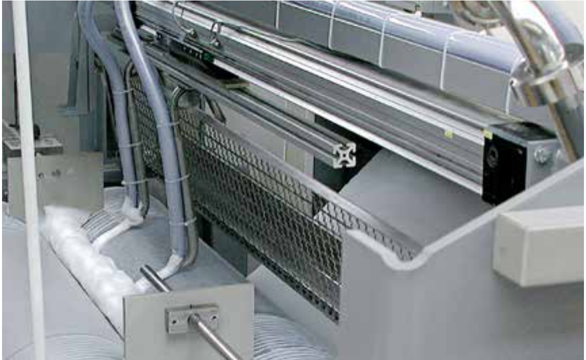
Impregnating by means of foam foulard
