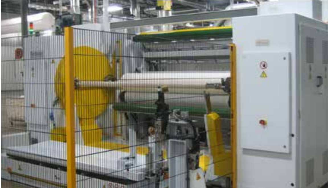
Automatic turret disc winder TWW-TD
