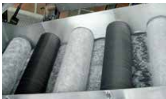
High random layer due to optimal arrangement of rolls
