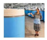
Even fully loaded – with up to 83 kg card sliver – the JUMBO CANS can be moved very easily over straight hall floors.
