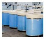
The 43% longer runtimes of the JUMBO CANS in the creel results in reduced downtimes on autoleveller draw frames or lap winders.
