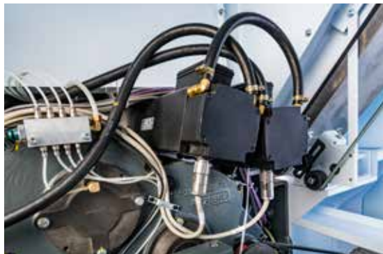
Two highly dynamic servo motors on each drive side.
