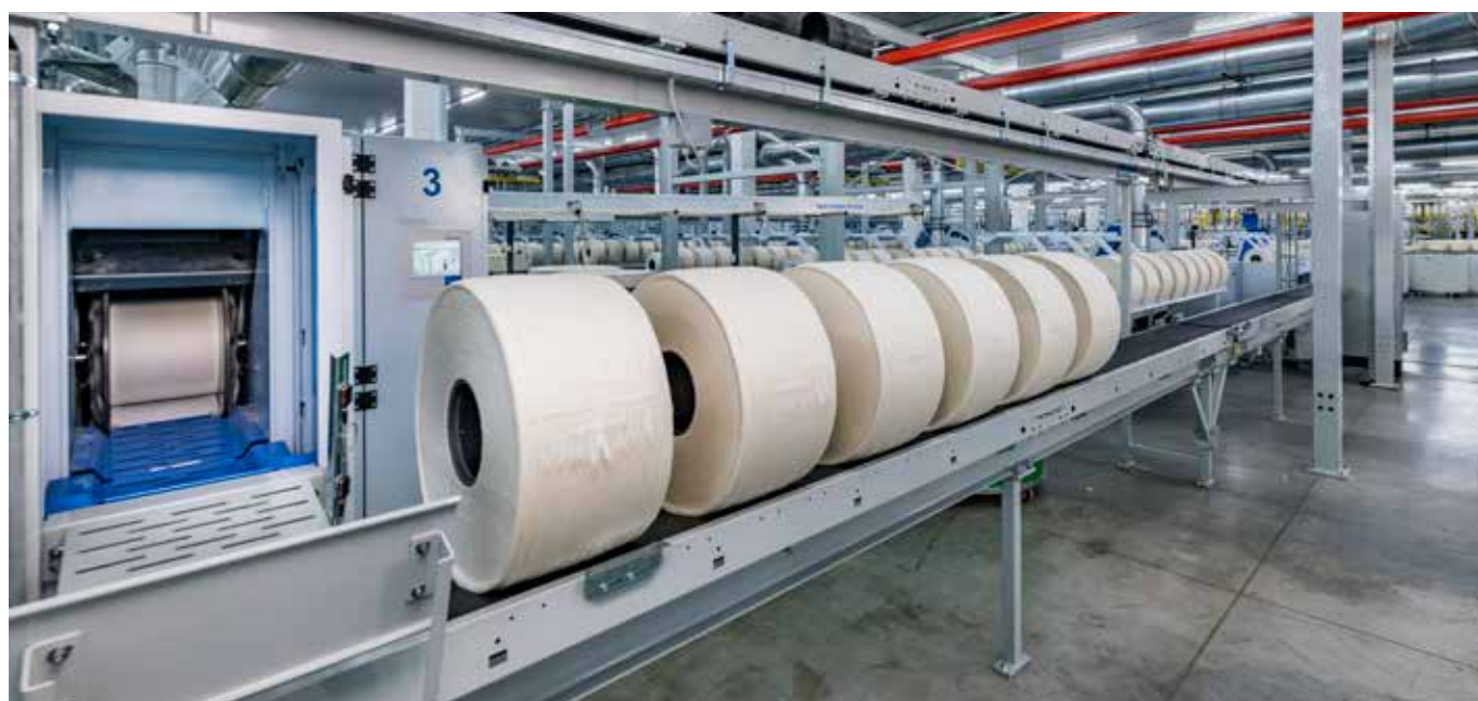
The picture shows the lap transport unit of the lap transport automation (LTS).
