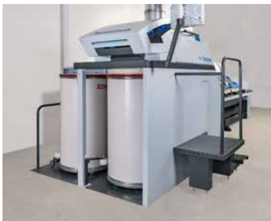
Below-floor variant. No ramp. Easier can handling.
