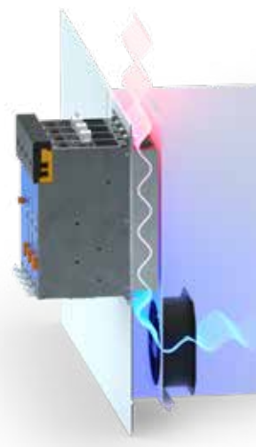
Intelligent control cabinet cooling, which leads to an increase in the service life of the electronic components.
