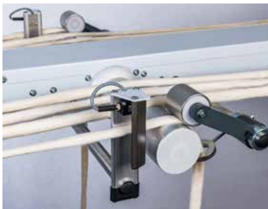
Individual sliver sensor in SMART CREEL
