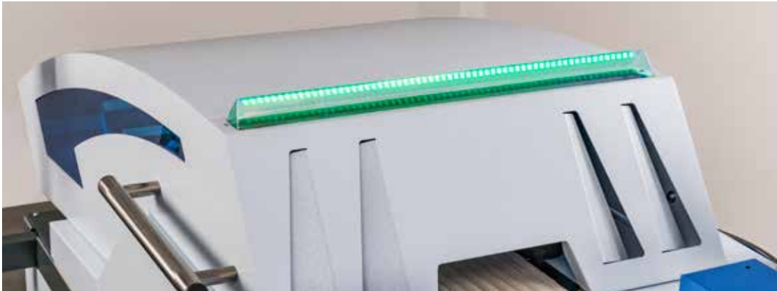
The remote display T-LED brings more overview to combing.
