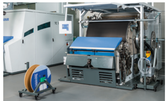
With the comprehensive Trützschler Mounting Equipment TC-ME, all cards are optimally prepared for clothing and re-clothing.
