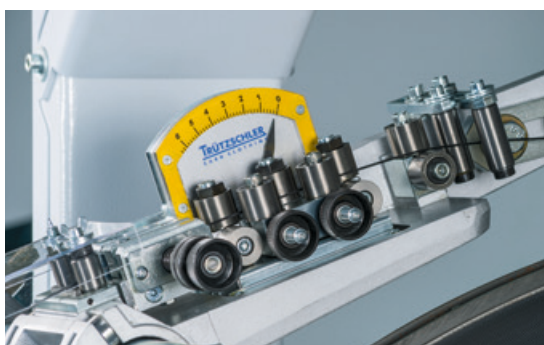
The corresponding T-Winder allows uniform mounting of any clothing type and thickness.
