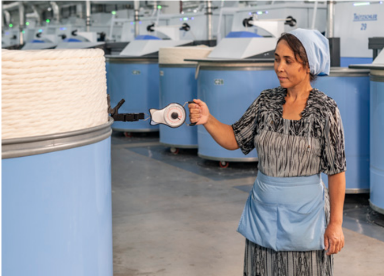
This JUMBO CAN contains 79 kg of card sliver. The test with the hanging scale shows that no more than 6-8 kg of force is required to move the can.
