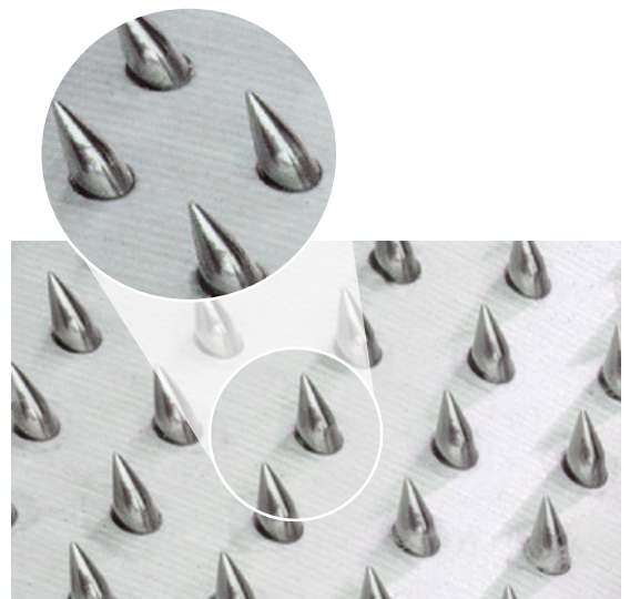
Needle licker-ins offer a long service life and are virtually maintenance-free
