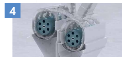
4 Guided material flow allows production of up to 2.000 kg/h
