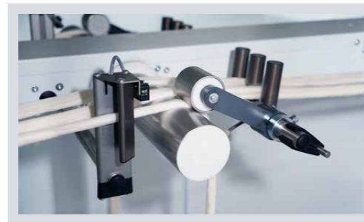
SMART CREEL sensors for individual sliver monitoring.
